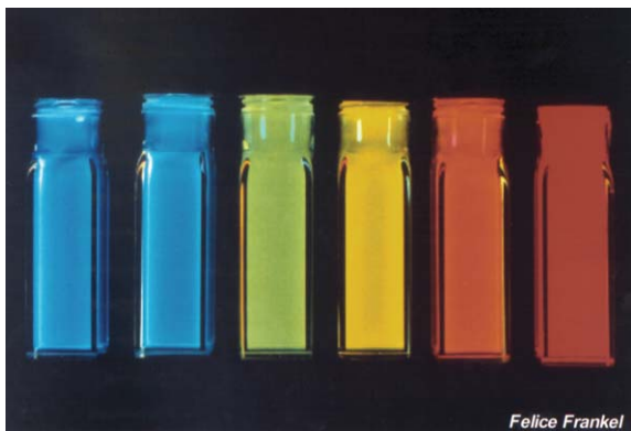
Fig. 1 Size-dependent emission properties of highly luminescent CdSe/ZnS NCs. From left to right, solution emission maximums are at 470, 480, 520, 560, 594, and 620 nm. Photograph by Felice Frankel. Quartz cuvettes courtesy of Spectrocell Inc. (Reproduced with permission from J. Phys. Chem. B , 1997, 101 , 9463. 3 Copyright 1997 American Chemical Society.)
